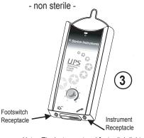
Note: The instrument and footswitch lights will not illuminate until the ENTceps are activated.
