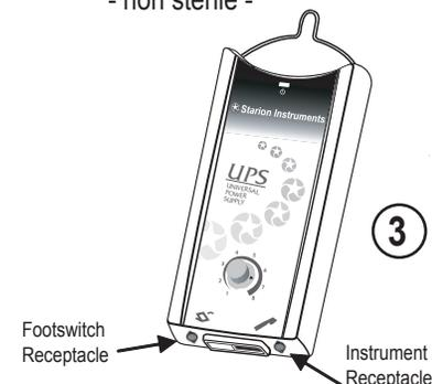
**Note:** The instrument and footswitch lights will not illuminate until the ENTceps are activated.
