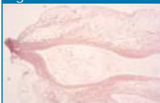
Photomicrograph of 2mm porcine gastroepiploic vessel welded shut with Starion laparoscopic device. Weld is darker upturned crimped area to the left. Magnification is 50x.
